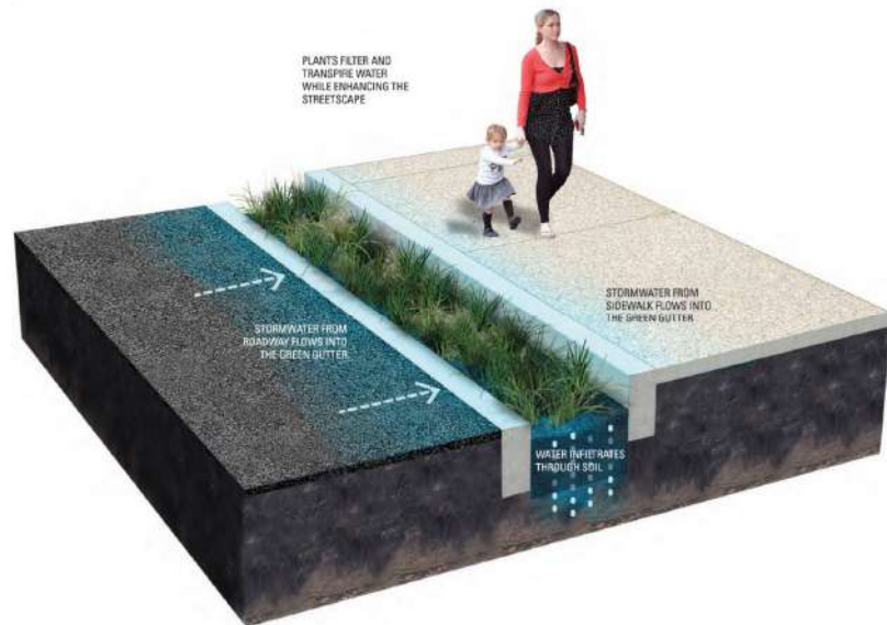
Green Gutter, Philadelphia, USA
